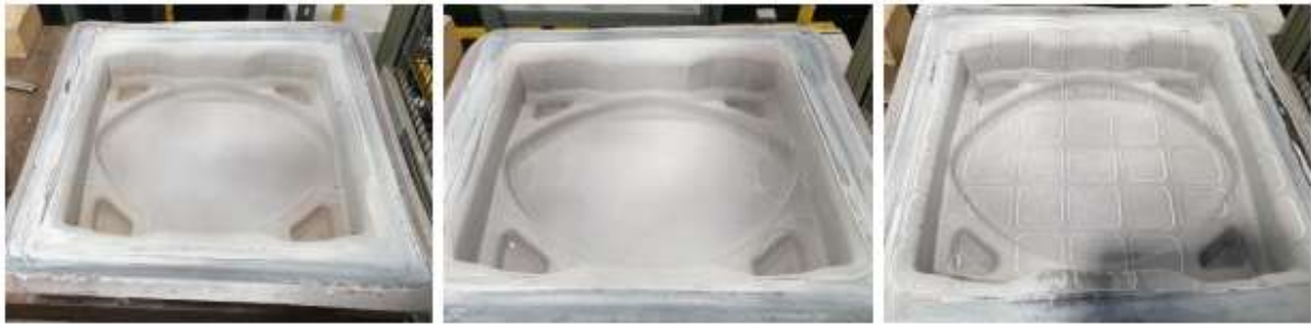
Figure 1 - Three tailored blanks that were designed and formed at the Advanced Forming Research Centre
